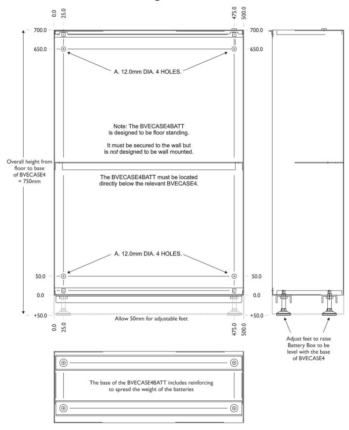
Note: The Adjustable feet should be set to raise the BVECASE4BATT to the level of the BVECASE4 installed directly above it.
