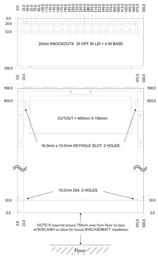
Note: The BVECASE4 has been designed to allow cable entry from the top (via knockouts) or via the removable access plate in the rear panel.
