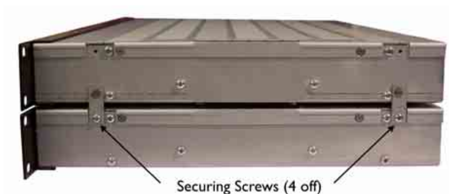
Figure 2.3 — Securing Slave to Master Unit
